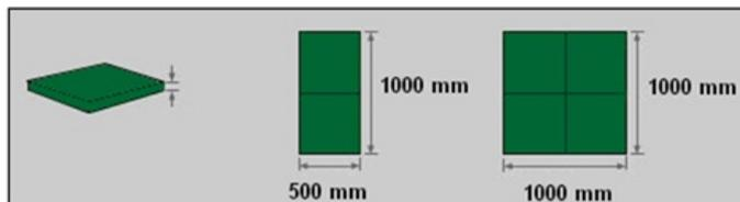
They are according to EN-1177. Critical fall height 1.83 m (HIC). Tested in the central testing laboratory IBV (Institute of Biomechanics of Valencia). **40 mm thick tiles are suitable for playgrounds.** 20 mm thick tiles do not comply with HIC standards for children's playgrounds.
